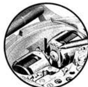
TO REGULATE 2 SECONDS PER DAY SLOWER, EITHER REGULATOR IS MOVED ONE DIVISION OUTWARD AS SHOWN.
