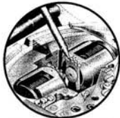
TO REGULATE 2 SECONDS PER DAY FASTER, EITHER REGULATOR IS MOVED ONE DIVISION INWARD AS SHOWN.
