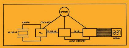
pulses are fed through two tiny solid state computer logic circuits which send electronic signals to the TELETIME display. These signals bring about a molecular change in the liquid crystal display material, causing sections of the display to become visible. These visible sections form the digits of the correct time on the display. The colon pulses once each second, while the proper digit or digits change each minute.
