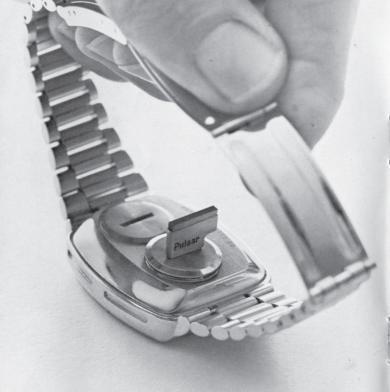
In the chamber nearest the command button, the "plus" sign on the cell should face up; the other cell faces "plus" side down. While doing this, be careful not to let one power cell touch the other, and be sure that each cell is properly seated in its chamber. Again using the timeset bar, screw the power cell hatches tightly into place.
